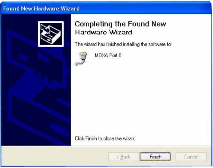
14. Repeat Step 7 through Step 11 for each of the remaining seven ports. The last port to be installed will be Moxa Port 7, as shown in the following figure.
