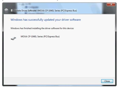
6. After installing the multiport serial adaptors driver, install the Moxa Port diver next. Right click on **MOXA communication port**. A popup window will open to help you install the driver for MOXA Port 0. Select **Update Driver Software...**
